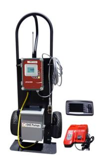
Recommended for full pipes and any fluid that contains solids or bubbles, the highly accurate UFL1000 powers, monitors, and displays the material flow rate in real-time. The wireless doppler ultrasonic flow meter display mounts securely in the cab of the heavy-duty machinery, providing complete data to the operator.
