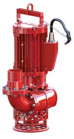
The Pump can handle up to 2.65 sp. gravity of solids & 70% by weight CW. This is subject to d50 values and calculation as per HI recommendation slurry pump selection procedure
